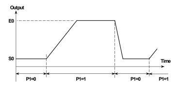
Both plots show a ramp on output J2, controlled using input P1 (on connector J7).
